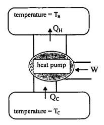
$Q_C$  = heat extracted from the cooler reservoir
