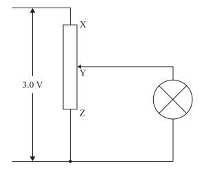
The potential divider XZ has a potential of 3.0 V across it. When the contact is at the position Y, the resistance of XY equals the resistance of YZ which equals 12  $\Omega$ . The resistance of the lamp is 4.0  $\Omega$ .
