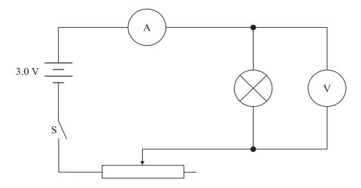
The supply is a battery that has an e.m.f. of 3.0 V and the ammeter and voltmeter are considered to be ideal. The lamp is labelled by the manufacturer as "3 Volts, 0.6 Watts".
