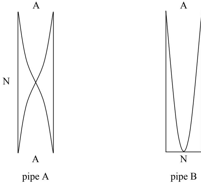
(i) correct wave shape for pipe A; correct wave shape for pipe B; [2]
