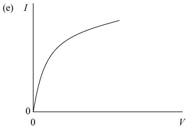
correct approximate shape (*i.e.* showing decreasing gradient with increasing  $V$ ); [1]
