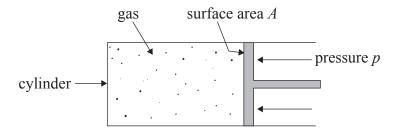
The piston has surface area A. A constant external pressure p acts on the piston.
