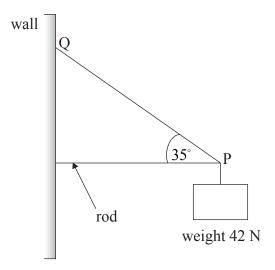
The rope makes an angle of 35° with the rod. The rod has negligible weight.
