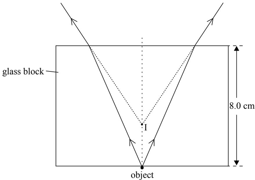
diagram showing correct refraction of one ray at surface;
