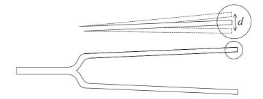
The extreme positions of the oscillating tip of one fork are separated by a distance d.
