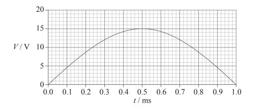
In order to convert this signal to a digital signal that can be stored on a CD, the signal voltage is measured at regular time intervals. The measured value is then converted into four-bit binary number by dividing the signal into 1 V levels.
