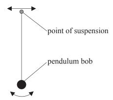
For each value of the driving frequency a steady constant amplitude A is reached. The oscillations of the pendulum bob are lightly damped.
