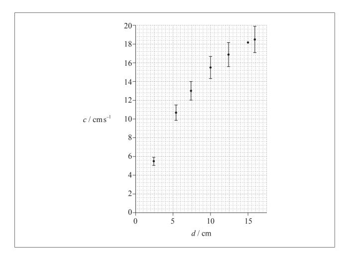
The uncertainty in the water depth d is too small to be shown. Uncertainties in the measurement of the wave speed c are shown as error bars on the graph except for the data point corresponding to  $d=15\,\mathrm{cm}$ .
