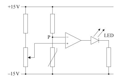
The amplifier operates from a  $\pm 15\,\mathrm{V}$  supply. If the thermistor reaches a certain temperature then, to act as a warning, the light-emitting diode (LED) switches on.
