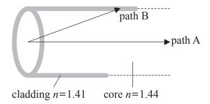
In a particular optic fibre of length  $2.00 10^4$  m, the refractive index of the cladding is 1.41 and that of the core is 1.44.
