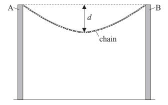
The length l of the chain can be increased by adding extra links. An experiment was undertaken to investigate how the sag d of the midpoint of the chain, measured from the horizontal between A and B, varies with l. The data obtained are shown plotted below. The uncertainties in l are too small to be shown.
