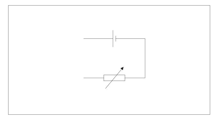
The variable resistor is set to  $1.5\Omega$ . When the cell converts  $7.2\,\mathrm{mJ}$  of energy, 5.8 mC of charge moves completely around the circuit. The potential difference across the variable resistor is 0.55 V.
