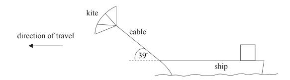
The tension in the cable that connects the kite to the ship is  $250 \,\mathrm{kN}$ . The kite is pulling the ship at an angle of  $39^\circ$  to the horizontal. The ship travels at a steady speed of  $8.5 \,\mathrm{m \ s^{-1}}$  when the ship's engines operate with a power output of  $2.7 \,\mathrm{MW}$ .
