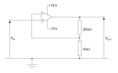
(a) (i) Calculate the gain of the circuit.
