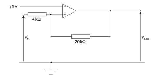
The output of the Schmitt trigger is positive saturation  $(+15\,\text{V})$  or negative saturation  $(-15\,\text{V})$ . Calculate the input value that will cause the output to switch from  $-15\,\text{V}$  to  $+15\,\text{V}$ .
