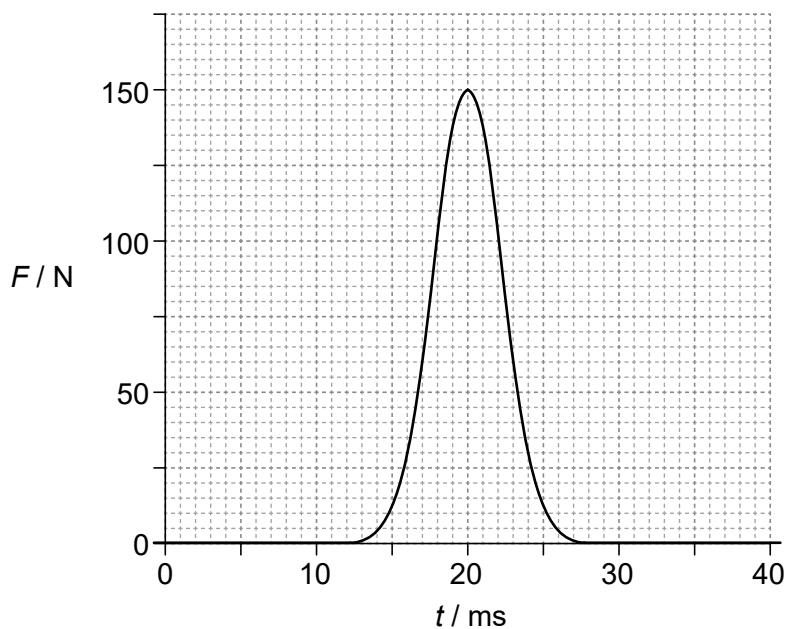
The tennis ball was stationary at the instant when it was hit. The mass of the tennis ball is  $5.8 \times 10^{-2} \text{ kg}$ . The area under the curve is  $0.84 \text{ N s}$ .
