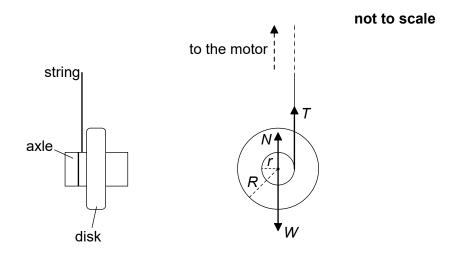
The moment of inertia of the flywheel about the axis is  $I = \frac{1}{2}MR^2$ .
